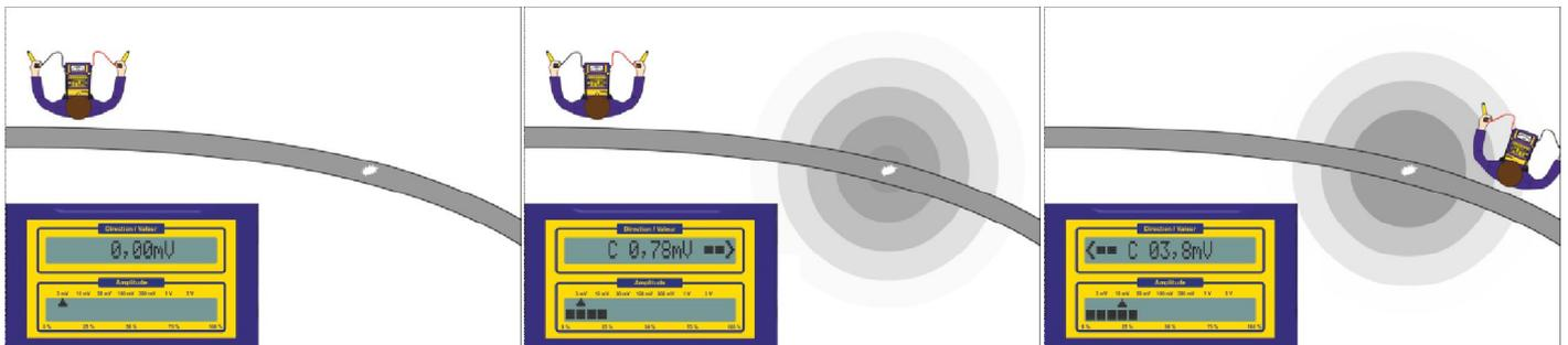
The operator goes back on his/her steps in order to find the point of equilibrium of the gradients, and the defect is identified in a first direction.
