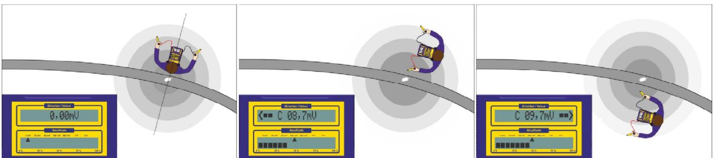
The two alignments then make it possible to draw a cross on the ground.
